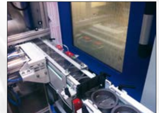
Feed conveyor for raw parts with baffle for prevention of false placed work pieces
