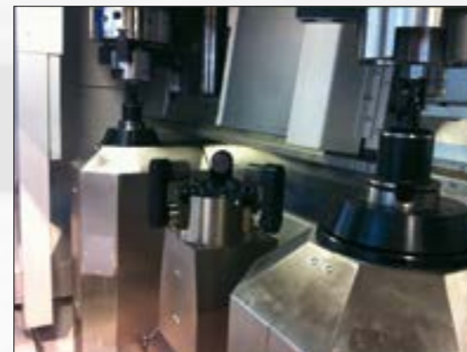
Simultaneous machining of clutch bodies at two processing stations of the machine DZS 315-2
