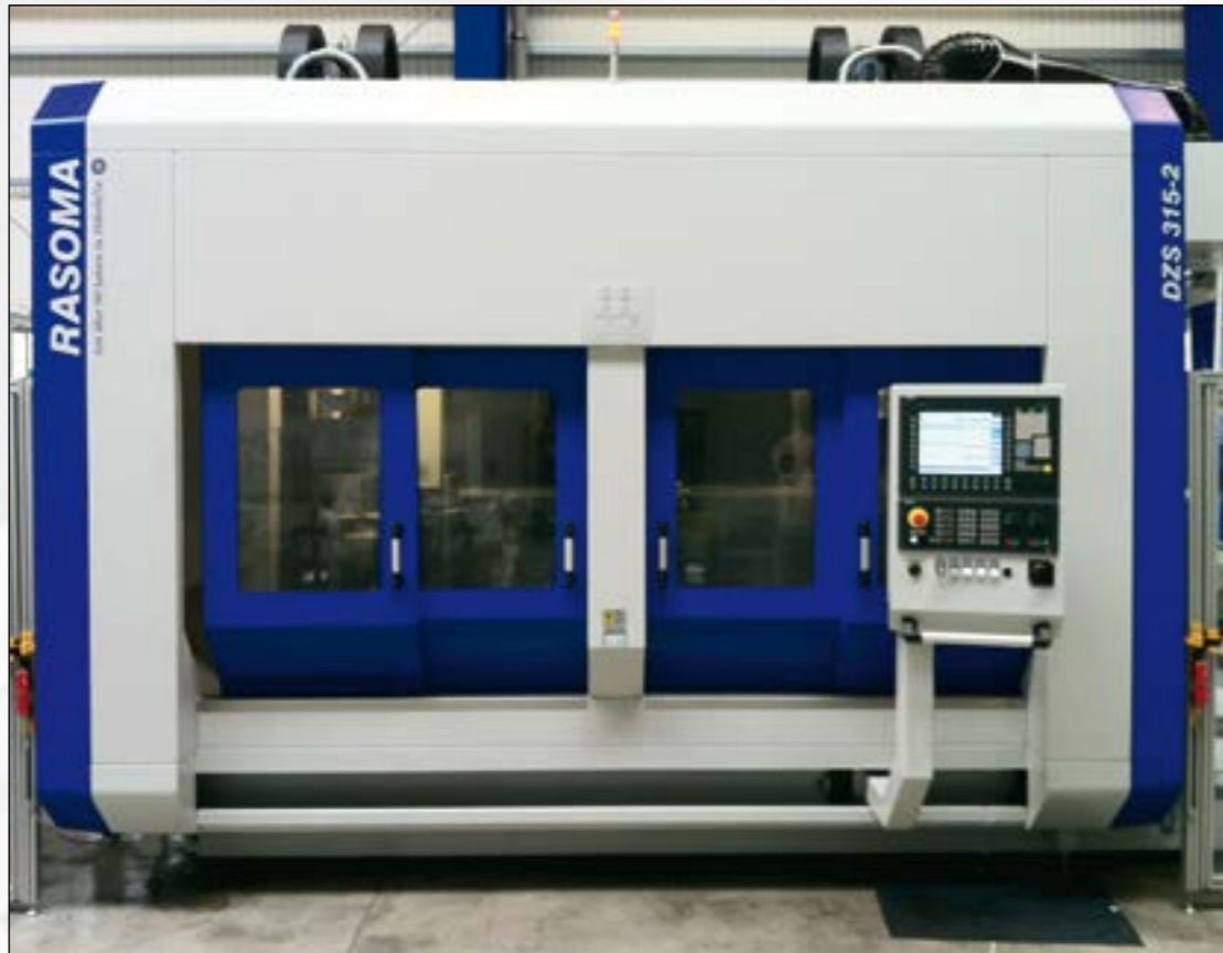
DZS 315-2 with 2 drilling-milling processing stations and 12-fold turret VDI 50
