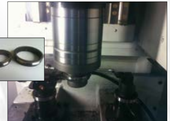
DZS 200-2 with block tools for synchronous processing of hardened sliding sleeves
