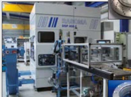
RASOMA special-purpose machine DSP 450-2 e.g. for perforating braking discs
