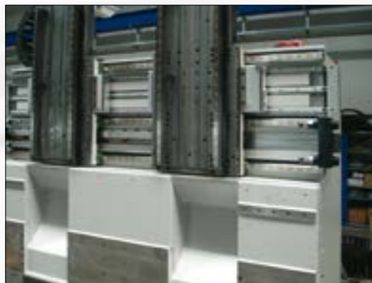
Basic structure of the DZS machines, here with two compound slides on three linear guides with intermediate linear motor
