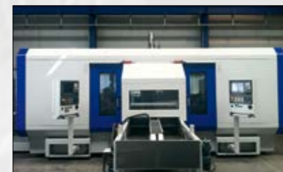
EBZ 60-900 with feed and discharge conveyor for work pieces through the center of the machine
