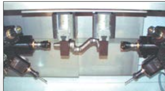
6-fold crown turret of EBZ 250-1000 for machining of crankshafts
