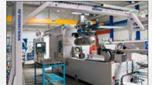
Loading and unloading of EBZ 250-1000 by the RASOMA linear gantry system with vertical axis and long stroke gripper with 36° module
