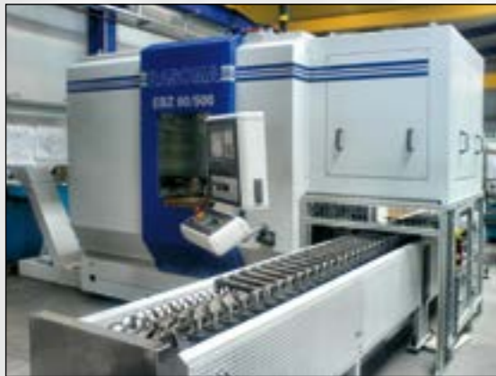
Rasoma end-machining centre EBZ 60-500 with permanent cycle conveyor for raw and finish parts
