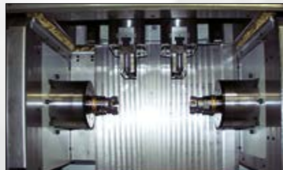
One motor spindle each for simultaneous machining of LH and RH side of the part
