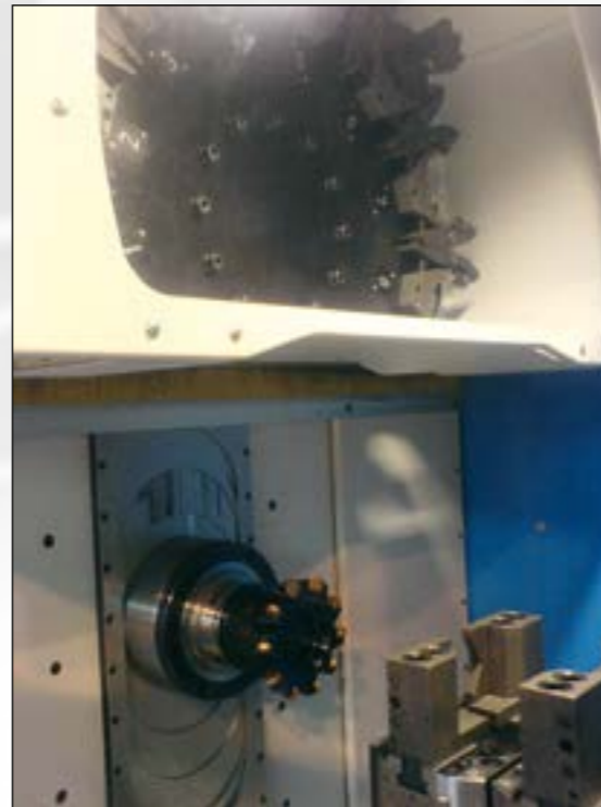
8-fold tool carrier on a three-axis module with spindle and face milling cutter of EBZ 250-1000
