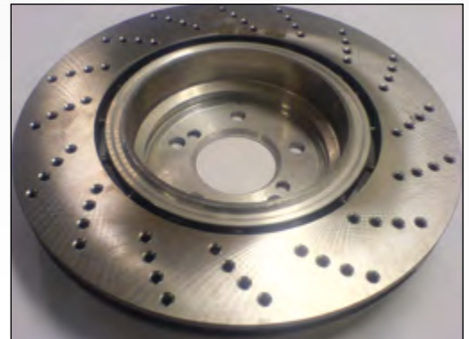
Perforating of brake disks: 0.25 ... 0.6 seconds per hole plus 9 seconds for automatic loading and unloading
