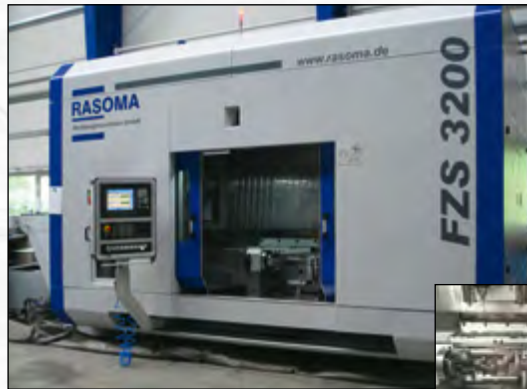
RASOMA manufacturing center FZS 3200 for end processing and oil drilling processing of crankshaft etc.
