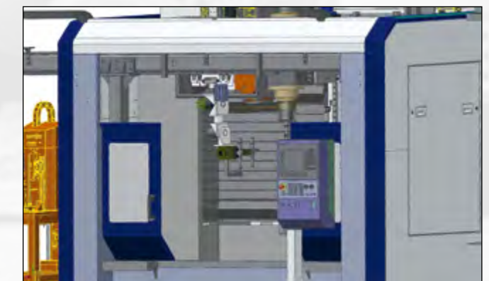
Principle of loading and unloading of shaft-type work pieces with machine-integrated RASOMA-articulated gantry loader
