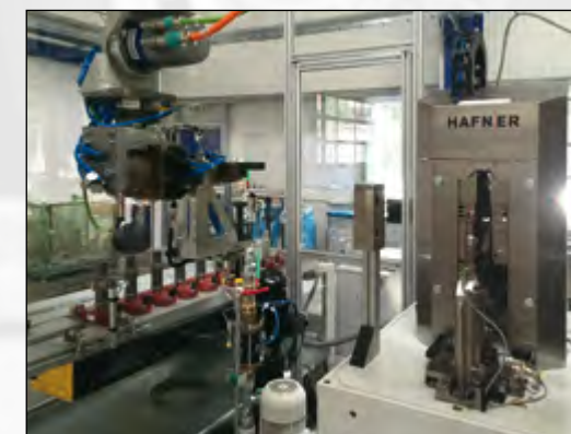
Machine-integrated RASOMA-articulating gantry loader and measuring station
