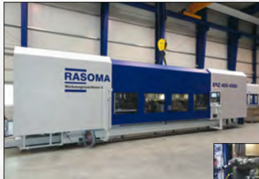
RASOMA end machining center EBZ 400-4500 for shaft-type work pieces up to 4,500 mm in length
